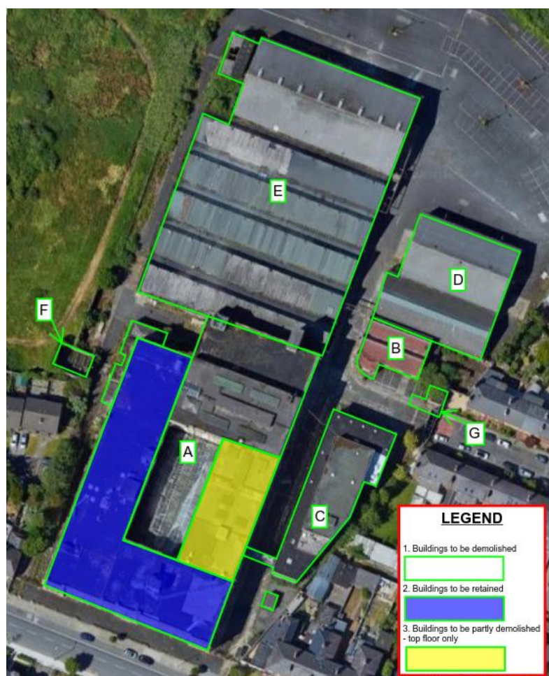
Figure 4.1 – Aerial view of site showing buildings to be demolished & building footprints.
